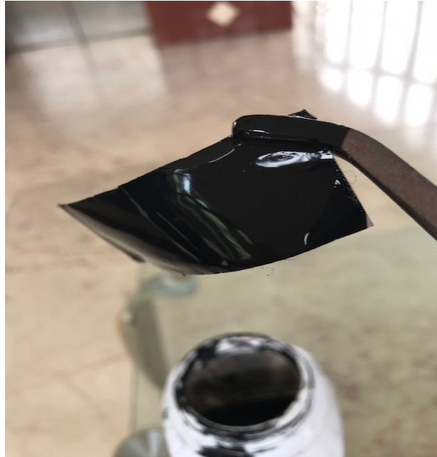
GRAPHENE Paint [Conductive] for supercapacitor metal sheet coating: High Surface area, High charge storage, Negative Electrode
